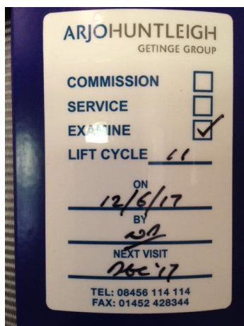
Examination sticker - hoist
